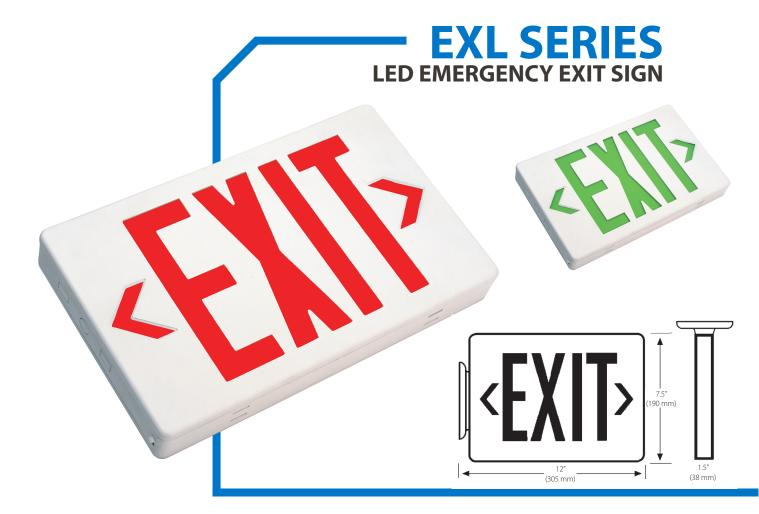
The EXL1 Series is a thermoplastic LED exit that combines a low-profile, contemporary design with the performance and dependability of LED technology in an affordable package. This series is available in white and offers universal mounting with testing button, Ni-Cad battery with low-voltage disconnection preventing deep discharge damage to the battery, and is also damp location listed. The EXL1 Series is a perfect modern-day, LED design for your project.
