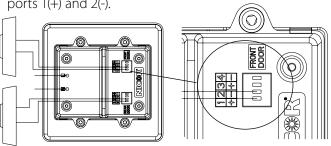
4 Install chime into junction box using four (4) included screws.
